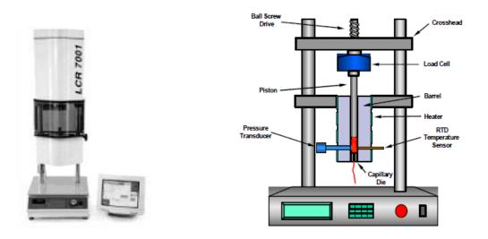
▶ A driven piston provides a constant volume flow (Shear Rate) or pressure (Shear Stress).
