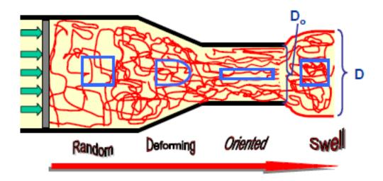
2. Swell decreases with an increase in temperature at a given shear rate or extrusion rate.
