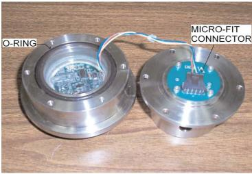
From the replacement kit remove the replacement sensor 'O'-Ring & package of grease. Grease the 'O'-Ring and place it in the groove. Attach the Micro-fit connector to PC board on the new adapter.
