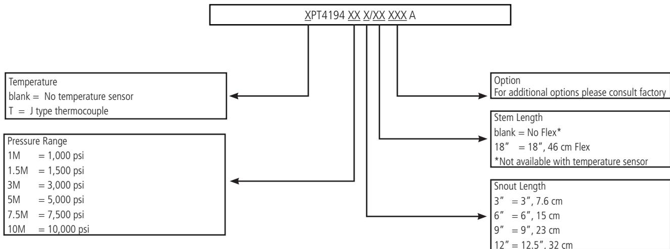
Standard mating connector Dynisco P/N 711600 or 6-pin mating connector cable assembly. Accuracy may be affected if non-standard configurations are used. For additional options please consult factory.
