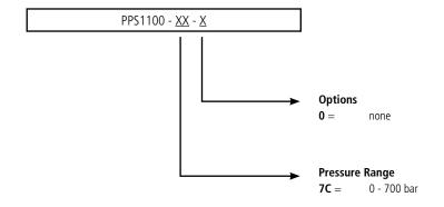
One adapter 1/2" 20UNF 2B is included at no additional charge. Other pressure ports on request.
