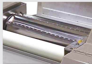
Cutting chamber with eight blade Pultrusion rotor.
