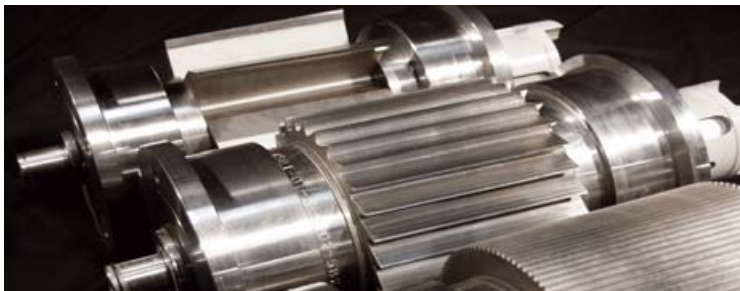
HM02F clamped tungsten carbide rotor (patented)
