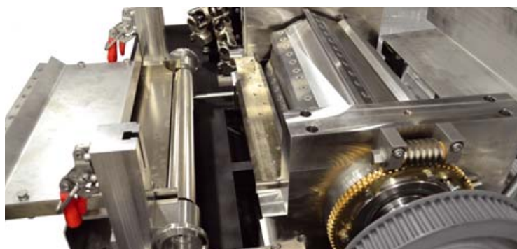
Sliding access to the cutting chamber for easy maintenance.
