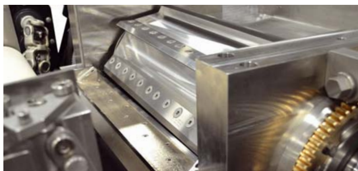
Cutting chamber with Eight blade Pultrusion rotor.
