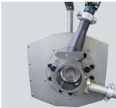
Wear-proof cutting Chamber
