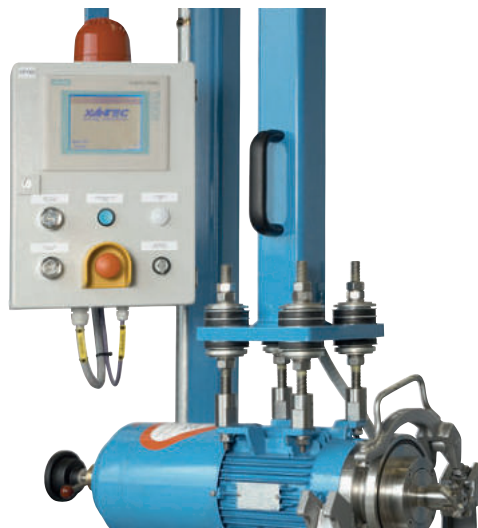
Operator panel with touch screen and Model MAP-5 Pelletizer
