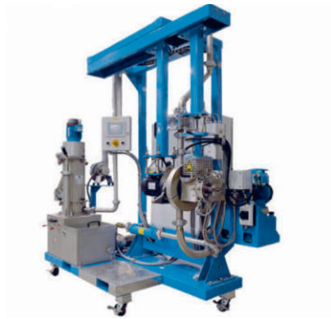
LPU™ with operator panel and SLC pelletizer
