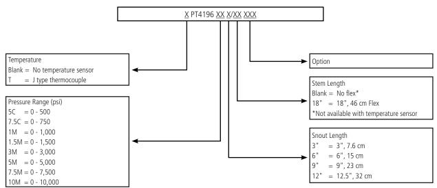
Standard mating connector Dynisco P/N 711600 or 6-pin mating connector cable assembly. Accuracy may be affected if non-standard configurations are used. For additional options please consult factory.
