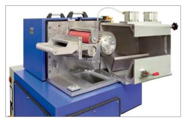
Throughputs up to 2.000 kg/h make the SGS 300-E6 the largest cantilevered strand-pelletizer available.
